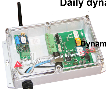
Internet controller with Wireless transceiver and precision temperature probe
